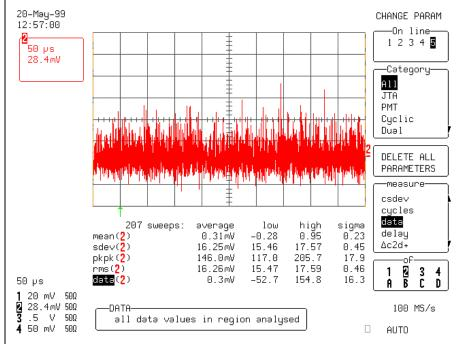
Figure 1-Characterizing a noise waveform in the time domain using parameter s
