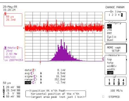
Figure 2 - Viewing the distribution of amplitude values using the histogram of the data parameter.
